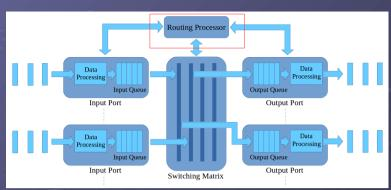
Routing processor: processes routing protocols, updates routing tables, maintains forwarding table used by input ports, monitors link state.
