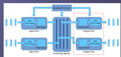
Output ports: retransmit received packet onto the selected out port.
