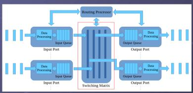
Switching matrix: connects an input queue/port to an output queue/port using crossbar, shared memory or bus etc. Connection determined by forwarding table in input port.
