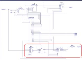
• A : all data buses and processing hardware increased to 16 bits e.g. data MUX, ALU, registers etc. University of York : M Freeman 2021
